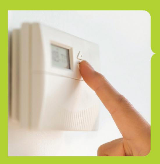
Adjust the thermostat to reflect occupied (21°) and unoccupied room temperatures (16°).
